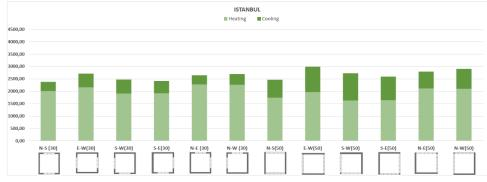
Figure 2: Annual heating, cooling and overall energy consumption for Istanbul
