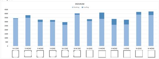
Figure 4: Annual heating, cooling and overall energy consumption for Erzurum
